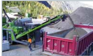
2. Production of mixture Nanoalps® System DRAIN with mixing machine
