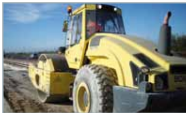
5. Compression of machined and improved road
