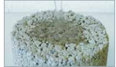
6. Demonstration of water permeability of final bound surface
